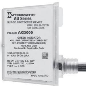
The AG3000 HVAC Surge Protective Device connects to the furnace/air handler disconnect to protect new high-efficiency furnaces, hydronic heating systems, air handlers, central air conditioners, wall-hung boilers, heat pumps and ductless mini-splits from surges. The Green LED indicates surge protection is present.
